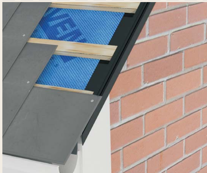
slate up the roof in the usual way
